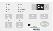
If the display reads "F4" a sensor has failed.
